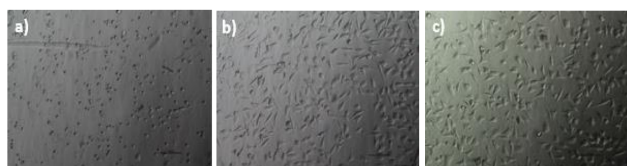
Figure 2: Direct Cell Contact Test on L929 mouse fibroblast: a) PCMS-Sty-40-VIm, b) PCMS-Sty-30-VIm c) PCMS-Sty-20-VIm
