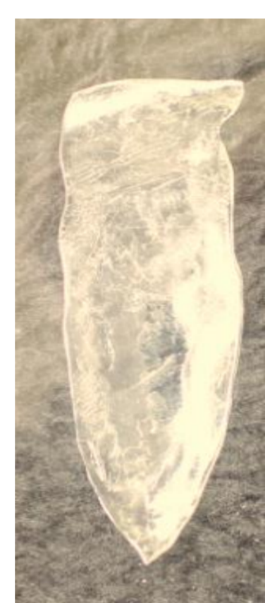
Figure 1: Film preparation: A solution of Polyelectrolyte 28 wt%, N-methyl-2-pyrrolidon 72 wt% and 2-Hydroxy-2-methylpropiophenone as a photoinitiator was cast with a 200 \mu\text{m} casting knife and irradiated with UV-light for 6 min.
