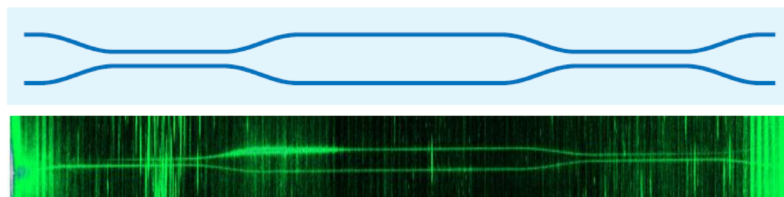
Fig. 1: Scheme (up) and fluorescence picture in false color (down) of an integrated optical Mach-Zehnder interferometer.
