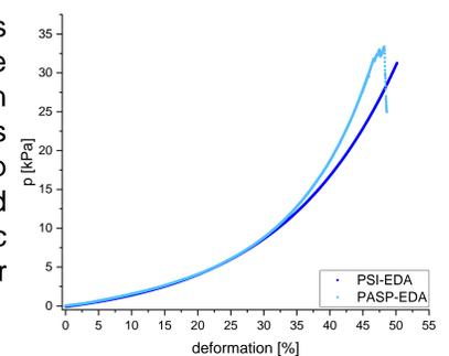
Figure 4: Comparison of the mechanical properties of PSI- and PASP-EDA-hydrogels.
