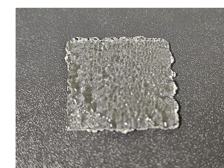
Hydrogel layer on silanised glass
