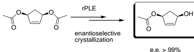
Figure 1. rPLE-catalyzed synthesis of enantiopure (1*S*,4*R*)-4-hydroxy-2-cyclopentenyl acetate.
