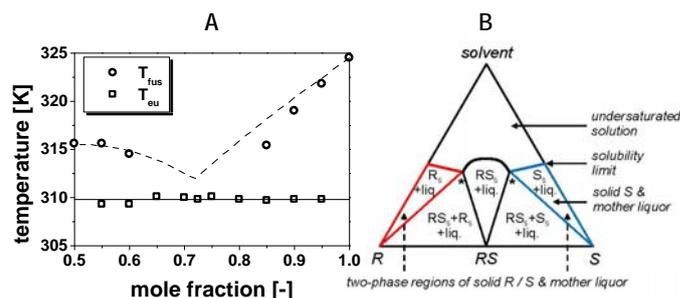
Figure 3. A) Binary melting point diagram of (1*S*,4*R*)-4-hydroxy-2-cyclopentenyl acetate. Theoretical calculation of the liquidus and solidus curve was performed applying the simplified equations of Schröder-van-Laar and Prigogine-Defay. B) Schematic representation of the ternary solution phase diagram of a racemic compound; \* - eutectic(s), R<sub>S</sub> - solid *R*-enantiomer, S<sub>S</sub> - solid *S*-enantiomer, RS<sub>S</sub> - solid racemic mixture, liq - liquid
