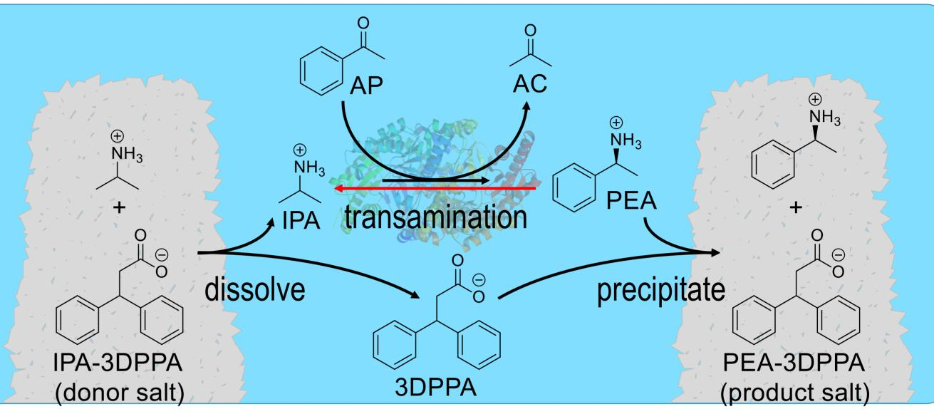
Fig. 1: reaction scheme for ISPC in transaminase-catalyzed reactions using donor salts
