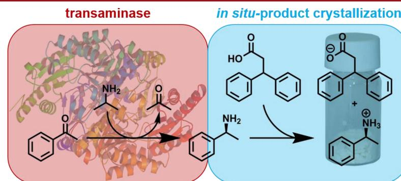
Fig. 1: crystallization-based *in situ* product removal in an amine transaminase-catalyzed reaction
