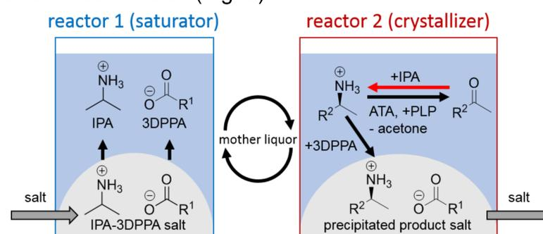
Fig. 3: process concept for a coupled two reactor system
