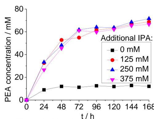
Fig. 2: fed-batch experiment using 125 mM IPA-3DPPA and 100 mM acetophenone (+ 10 mM every 24 h), pH 7.5, 30 °C, 1.5 U·mL<sup>-1</sup>
